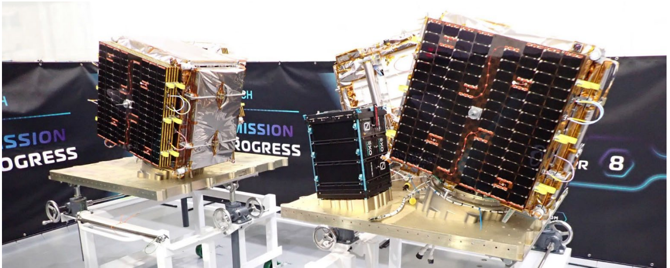
Figure 6: Four CarboNIX 15s sharing a plate with EXOpod Novas and ready to launch on Transporter-8.
