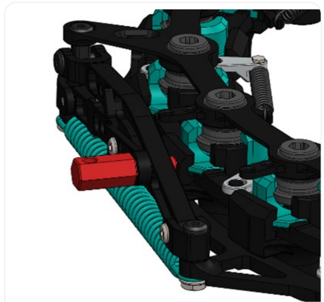
Figure 28: Pushing Mechanism RBF Binds Two Arms Together and Prevents Deployment.
