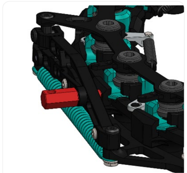
Figure 28: Pushing Mechanism RBF Binds Two Arms Together and Prevents Deployment.
