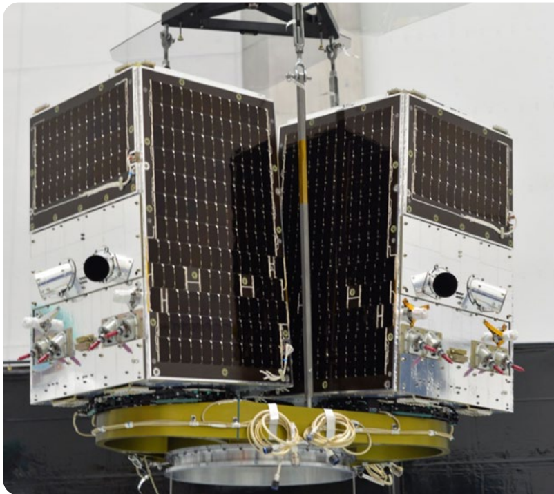
Figure 4: Three CarboNIX 15 units were used on the June 13, 2020 SpaceX Starlink-9 Rideshare Mission. Each SkySat had a mass of 110 kg.
